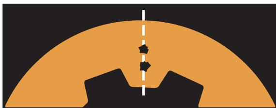
Cross-section showing portion of corrosion (leak)
